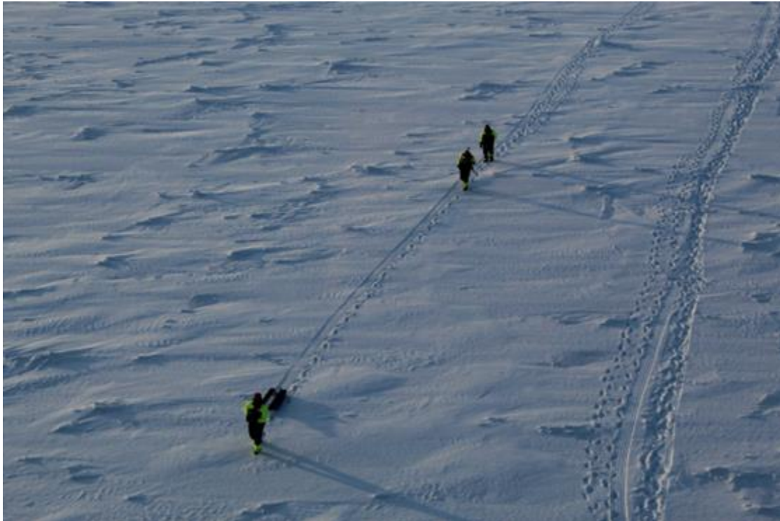
Figure 2: Conducting snow and ice thickness survey using GEM-2 and Magnaprobe instruments. A person in the front pulls a sled with the EM instrument (in this case GEM-2). Snow thickness measurements along the same track are conducted using the MP instrument by another person that keeps the distance from the EM operator to ensure the electromagnetic measurements are not biased by proximity of large metal objects. Photo taken during the Seasonal Q1 cruise, Station P5 on 12.03.2021. Photo: S. Gerland (NPI).
